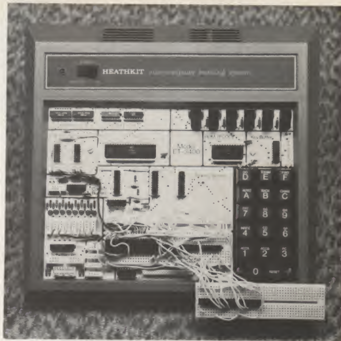
Photo 2. Trainer close-up with breadboard circuitry.
